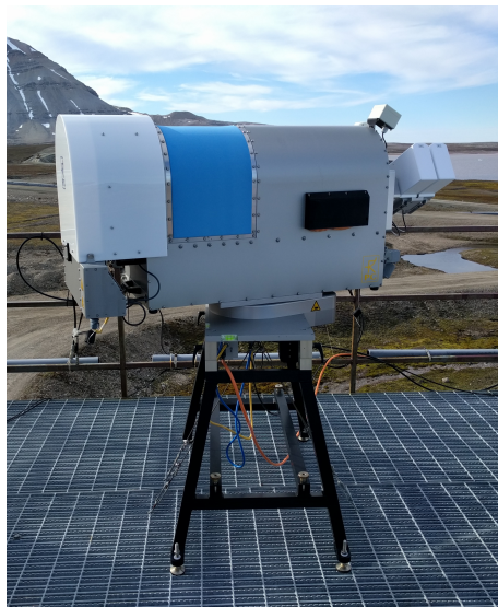
Figure 2.3: MWR HATPRO mounted on the roof of the AWIPEV station at Ny-Ålesund.
