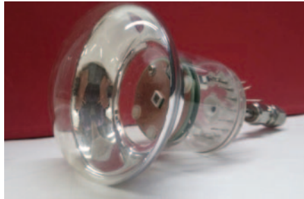
Fig. 4. – A picture of the 3-inches prototype, taken during one of the mechanical tests on the device.
