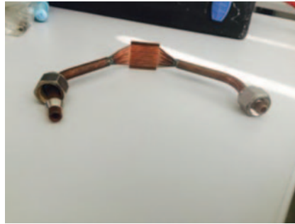
Fig. 2. – Target used for the tests. The beam impinges on the part where tubes are accommodated in the backing.
