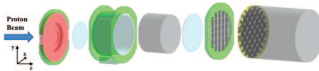
Fig. 1. – Dismanteled view of the main components of the spallation target as implemented in the Geant4 simulation.
