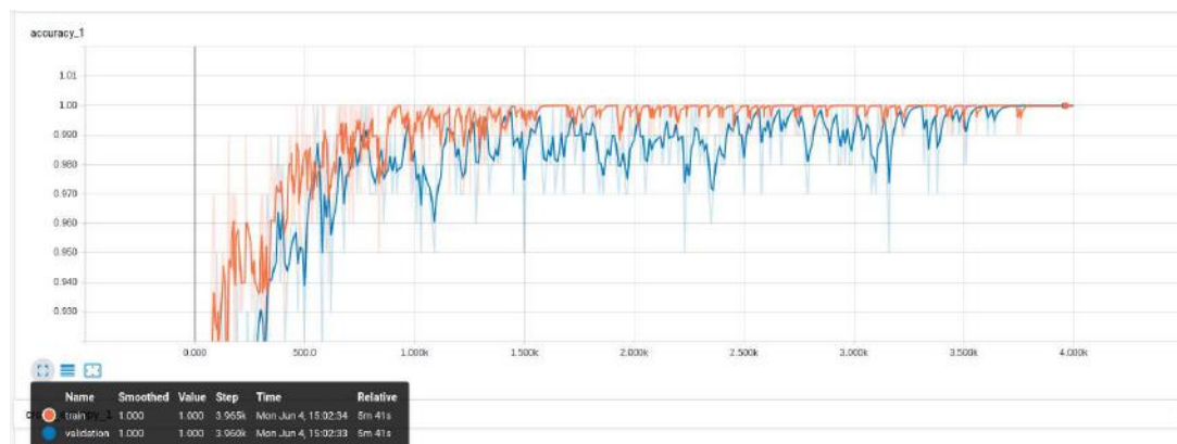
Figure 11. Illustration of the increase in the accuracy over the number of iterations. The training and the validation become stable after 3900 training steps.
