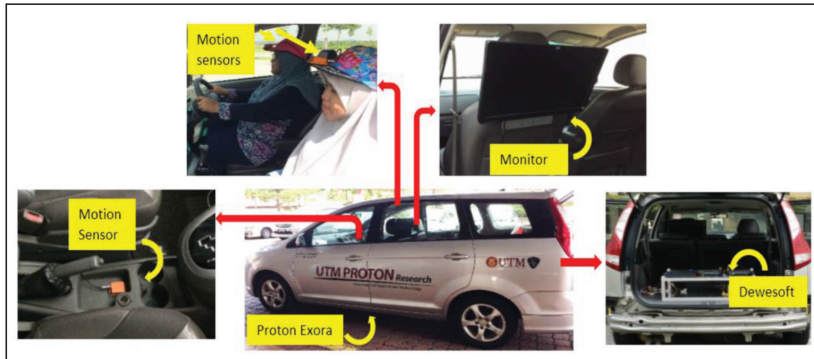
Figure 2. The placement of equipment installed in a Proton Exora.
