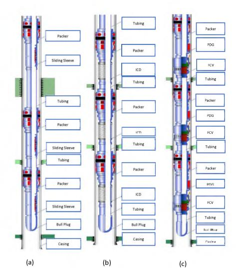
Figure 1.1 (a) Multi-zone with sliding sleeve, (b) Multi-zone with ICD, (c) Multi-zone with FCV and PDG
