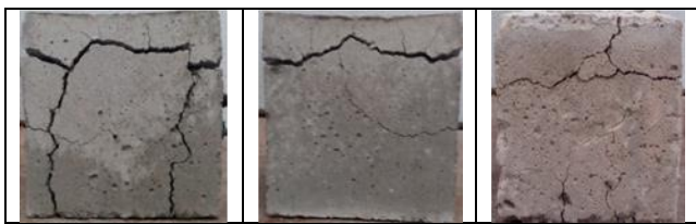
Figure 12 Surface texture of the sawdust concrete samples ratio 1:1, 1:2, 1:3 exposed to 800°C
