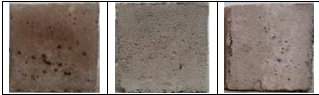
Figure 10 Surface texture of the sawdust concrete samples ratio 1:1, 1:2, 1:3 exposed to 400°C
