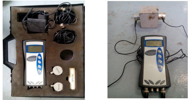
Figure 3 Ultrasonic pulse velocity (UPV) testing apparatus
