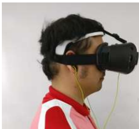
Fig 2.1: Experimental Setup with EEG headset and VR Headset
