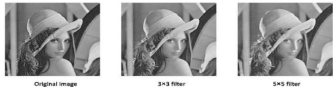
Fig. 4. The changes of Lena image when applying 3x3 and 5x5 maximum filters
