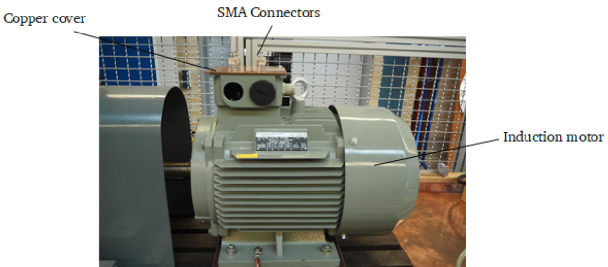
Figure 2.8.: The RF S-parameters measurements of the induction motor.
