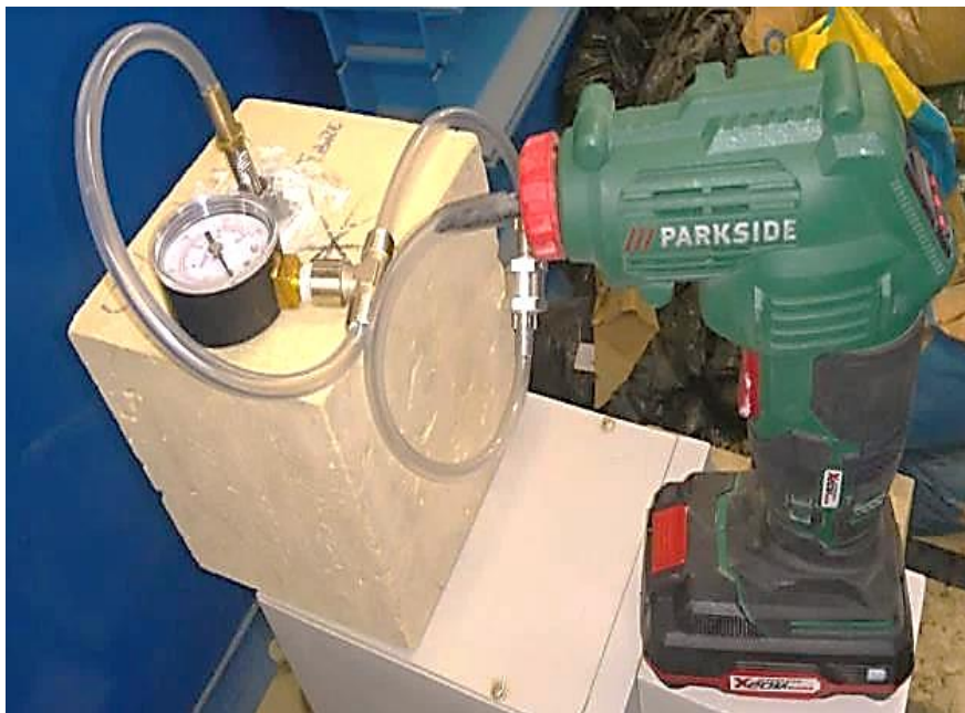
(b) Test apparatus attached to a portable pump.
