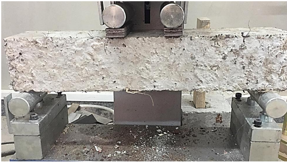
Figure 3: Setup of flexural strength test.
