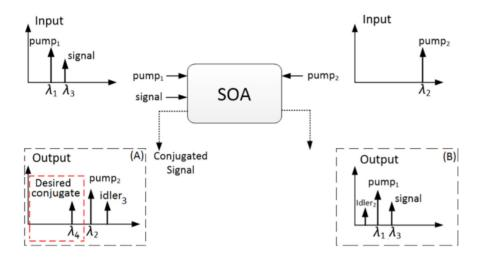
Fig. 1. Block-diagram of dual pumped counter-propagating FWM in SOA. Pumps are detuned from symmetrical position of signal to facilitate optical filtering of conjugate.  $\lambda_1$  and  $\lambda_2$ : forward and backward pump wavelength,  $\lambda_3$ : signal, and  $\lambda_4$ : conjugate wavelength
