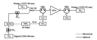
Fig. 2. Generation of phase conjugated wave using counter-propagating dual pumps in SOA.  $TL_{1,2,3}$ : tunable laser, MZM: Mach–Zehnder modulator, PPG: pulse pattern generator, CIRC<sub>1,2</sub>: circulator, SOA: semiconductor optical amplifier, OTF: optical tunable filter, OSA<sub>1,2</sub>: complex optical spectrum analyzer.
