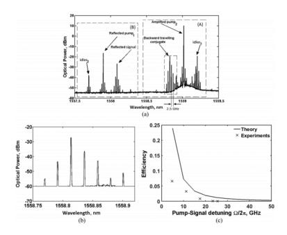
Fig. 3. (a) Spectrum of FWM products with input signal modulated by repetitive sequence of '1000' at 10 Gbps, (b) spectrum of backward propagating conjugate after filtering by OTF. Note flipping of spectrum at backward travelling conjugate (1558.83 nm) due to phase conjugation, and (c) dependency of conversion efficiency of backward travelling conjugate with detuning between pump1 and signal.
