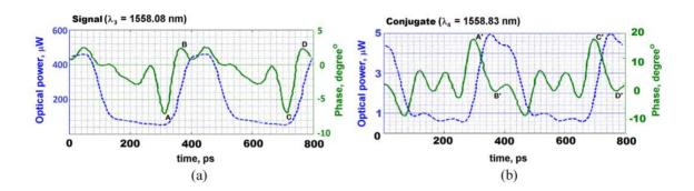
Fig. 4. Intensity and phase vs time plot of (a) input signal,  $\lambda_3$  = 1558.08 nm and (b) filtered output (conjugate),  $\lambda_4$  = 1558.83 nm. Dashed line – intensity. Solid line – phase. We observe phase inversion at bit transition AB–AB" and CD–C'D'.
