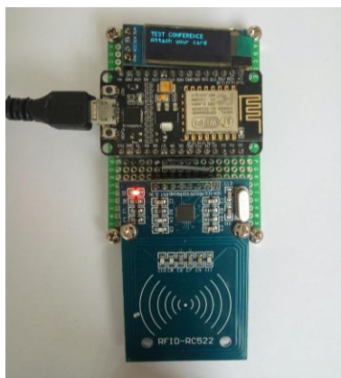
Figure 4. Model of controller with the NodeMCU development board
