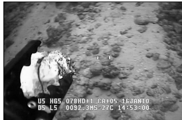
Figure 7. Using the manipulator arm to sample rhodoliths at 92 m (black and white image of a color video capture).
