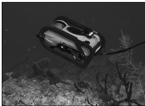
Figure 1. Seabotix 200 LBV remotely operated vehicle used for study of mesophotic coral ecosystems. ROV is shown hovering over the shelf break.
