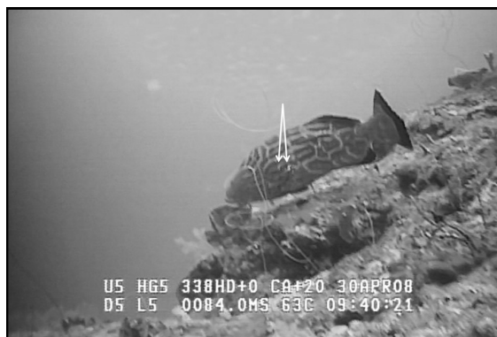
Figure 4. Measuring a black grouper at 84 m. Arrows point to the two parallel laser beams set 5 cm apart (black and white image of a color video capture).
