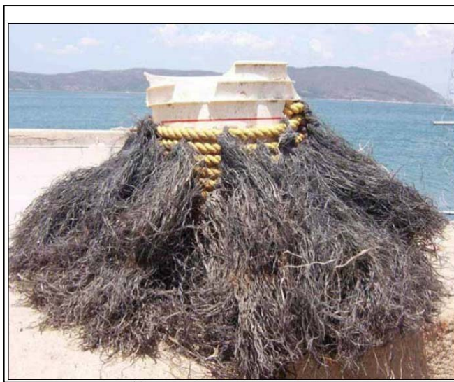
Plate 1. Modified GUSI lobster postlarval collector used in present study with central plastic bucket and teased-out black synthetic rope tassels forming “skirt” around bucket.
