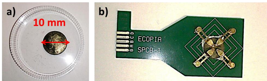
Figure 4-18: a) Illustration of the 10 nm diameter DPP2-HHTTP-COF pellet and b) construction of the Hall measurement setup in the van der Pauw geometry.
