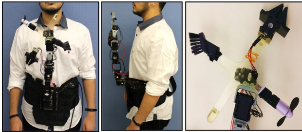
Fig. 2 Front and side views of HapticHydra. The multifunctional end effector is able to deliver multiple types of feedback as it is equipped with a gripper, a fan, a finger-shaped effector and a brush
