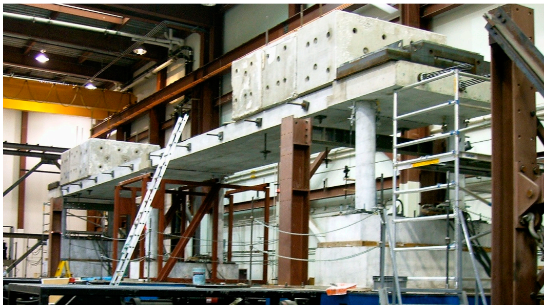
Figure 2. Experimental setup and sensor layout of the Bridge 1 test, conducted at University of Nevada, Reno [39].
