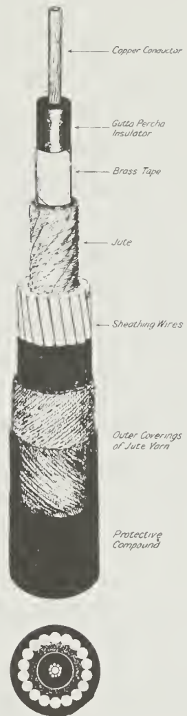
Fig. 38 Component parts of a typical deep sea telegraph cable.
