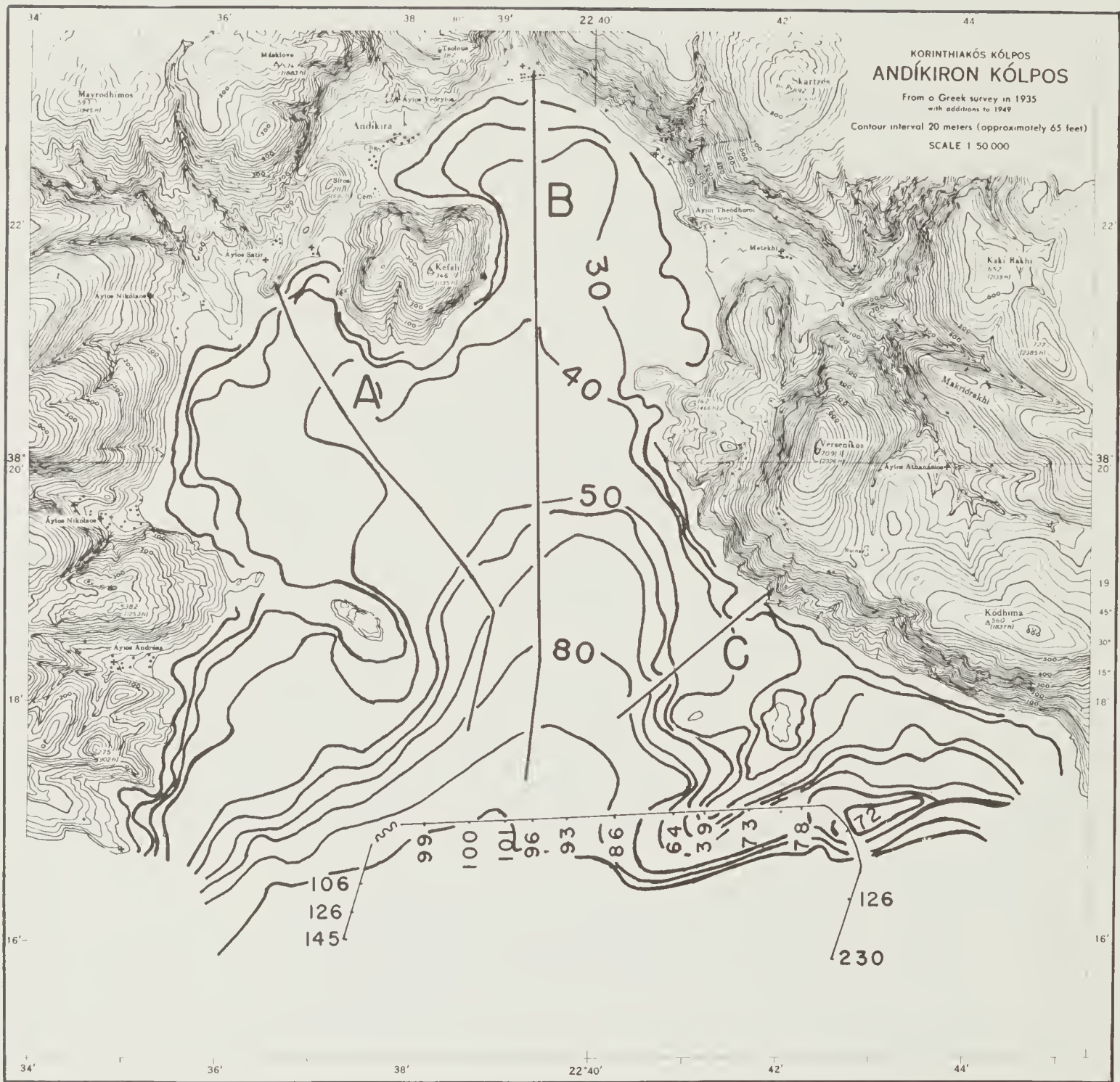
Fig. 10 Bathymetric sketch of the Andíiron Gulf. Andíiron Gulf after U. S. Hydrographic Office Chart 4092. Profiles A, B and C are shown in Fig. 9. Contour interval 20 meters (10.9 fathoms) on land, and 10 fathoms in Andíiron Gulf.
