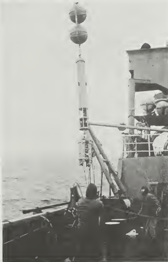
Fig. 3. Launch of a bottom-moored current meter array, Cruise 47.
