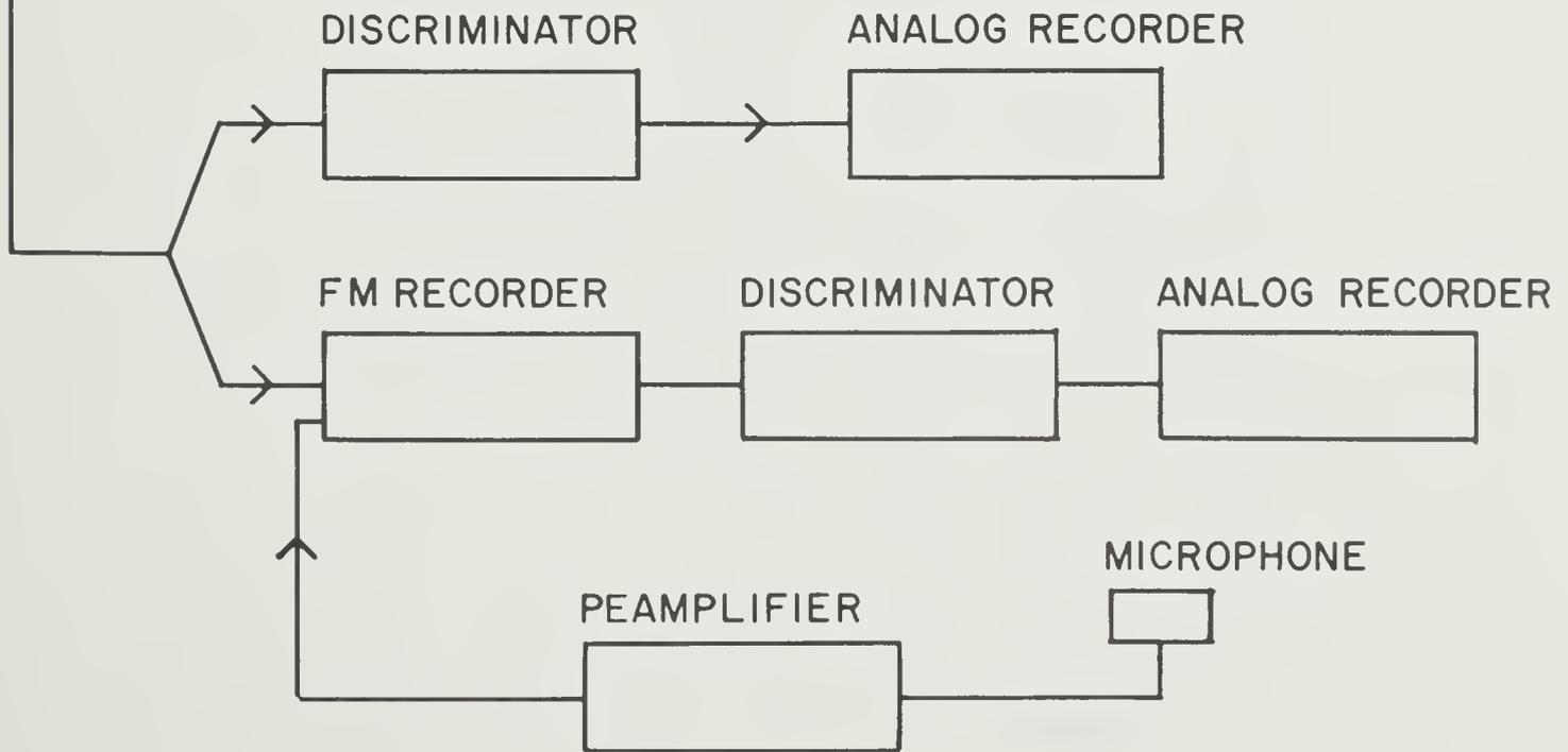
Figure 1. Projectile impact recording system block diagram - only one of three channels shown.
