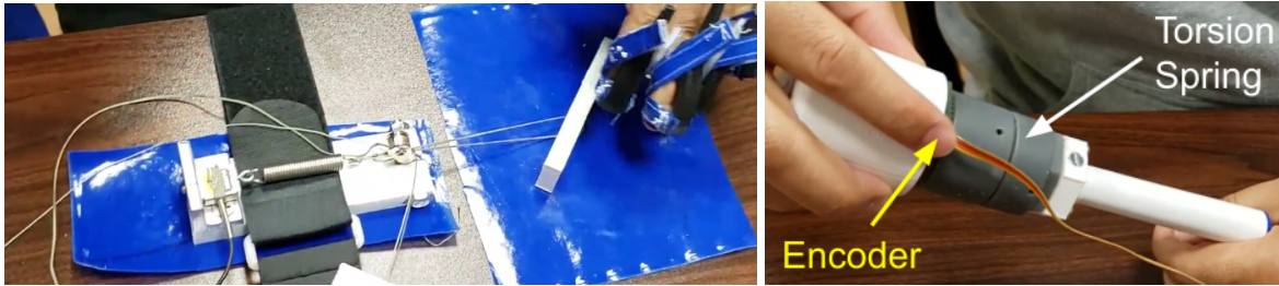
Figure 7.3: Weight measurement setup (left) and torque measurement setup (right).
