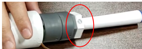
Figure 7.5: Torque measurement tool mounted with a marker. The subjects took advantage of the highlighted portion of the tool to increase stabilization force.
