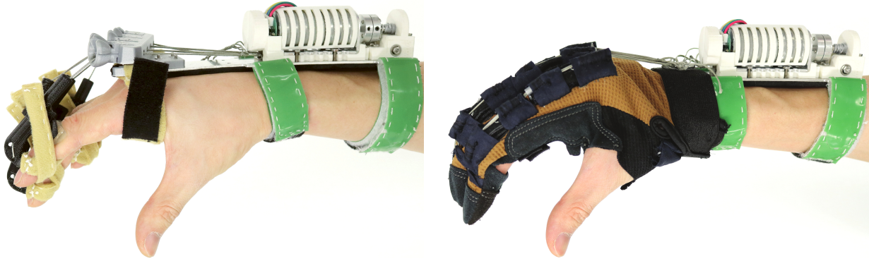
Figure 4.4: Prototypes of the hand orthosis transmission mechanisms (top: Design A, bottom: Design B) proposed in this study.
