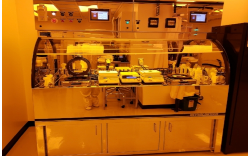
Figure 4.2: Hood equipped with spinners and hot plates for baking resist.
