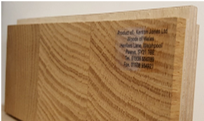
Figure 2: The “Inside-out beam” is a large-dimensioned beam derived from a small-diameter log. The process involves machine rounding the log, squaring the edges, sawing the log into four sections before gluing the rotated sections together again.
