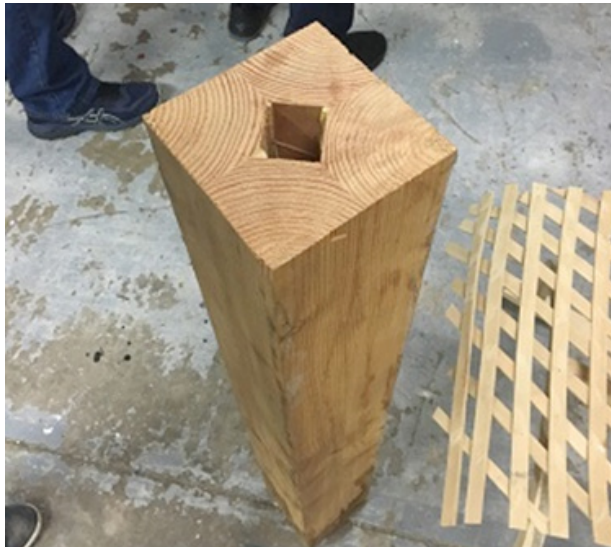
Figure 2: The “Inside-out beam” is a large-dimensioned beam derived from a small-diameter log. The process involves machine rounding the log, squaring the edges, sawing the log into four sections before gluing the rotated sections together again.
