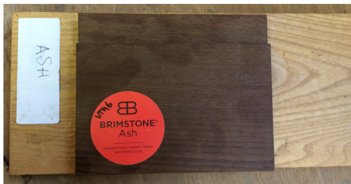
Figure 6: Brimstone ash weather cladding – a new heat-treated exterior cladding board developed by Vastern Timber – placed on an untreated ash plank for comparison.
