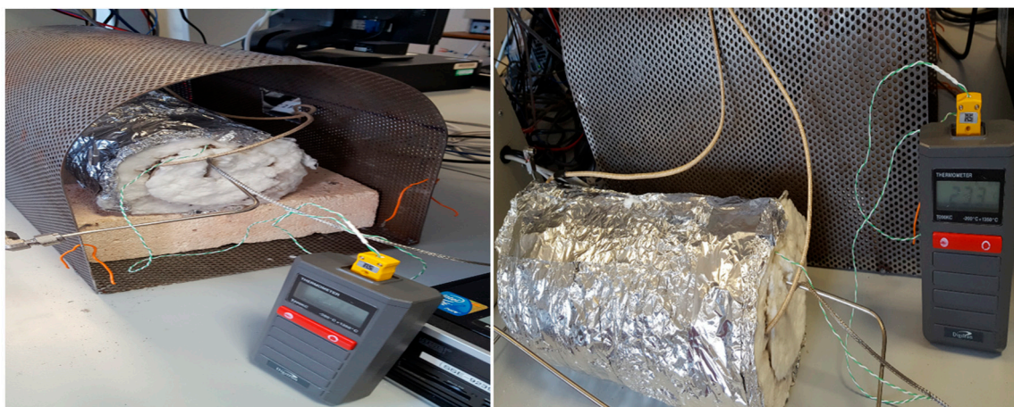
Figure 16. Tubular furnace sealed with ceramic fiber blanket with the microreactor inserted at the center of the furnace.
