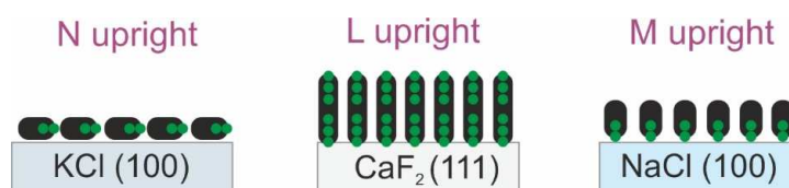
Figure 1: Substrate controlled orientation of 6F-pentacene 38b .
