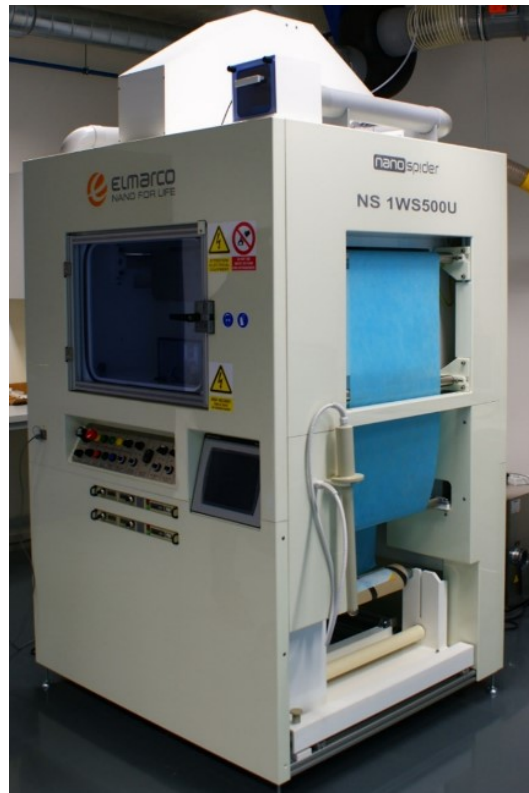
Figure 16: The Nanospider NS 1WS500U used in PCL fibre matrix preparation.
