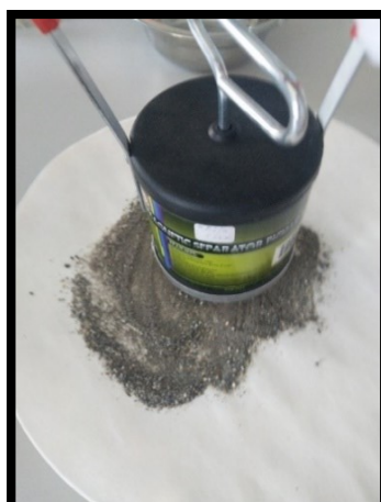
Obr. 24: Magnetic separator SE 16-lb
