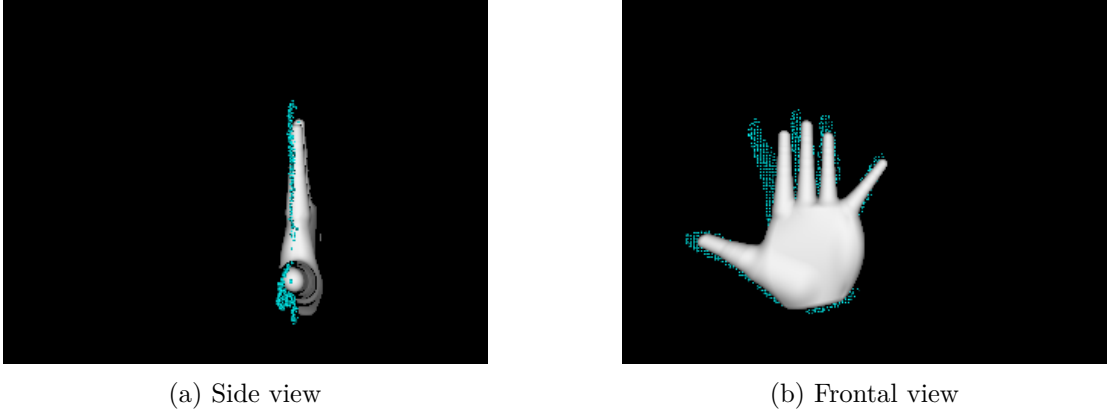
Figure 10: Rendering of the SDF model fitted the point cloud of segmented hand model
