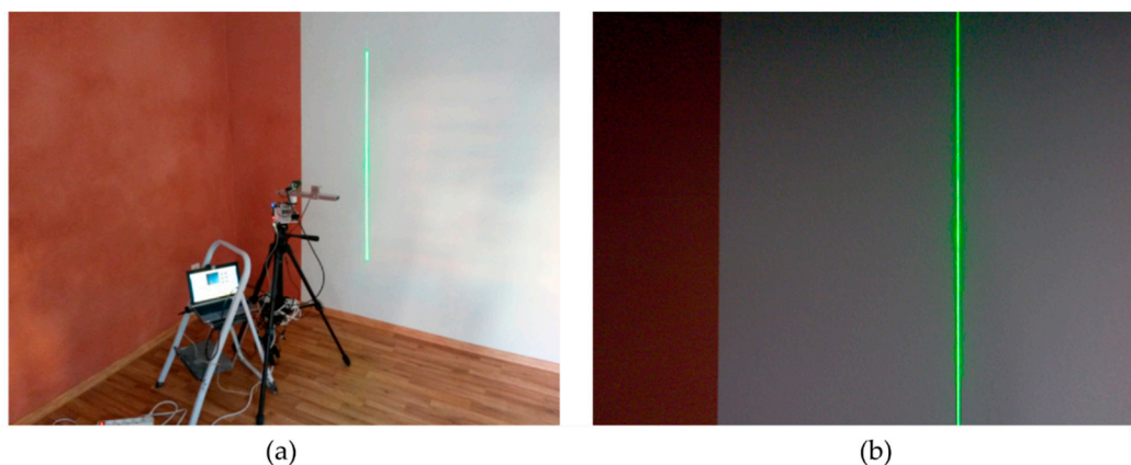
Figure 16. Measurement illustration: (a) Developed 3D scanner; (b) Measurement frame.
