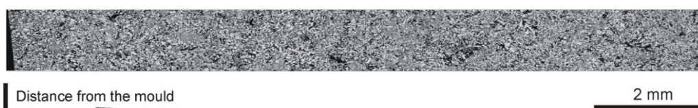
Figure 9. Microstructure evolution with distance from the wall of the mould in bottom part of W–Al–VIM-2 ingot.
