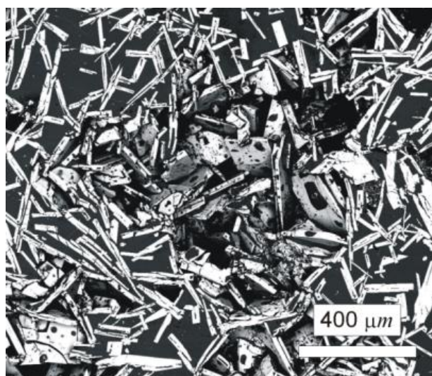
Figure 7. Shrinkage in the upper part of the W–Al–VIM-1 alloy.
