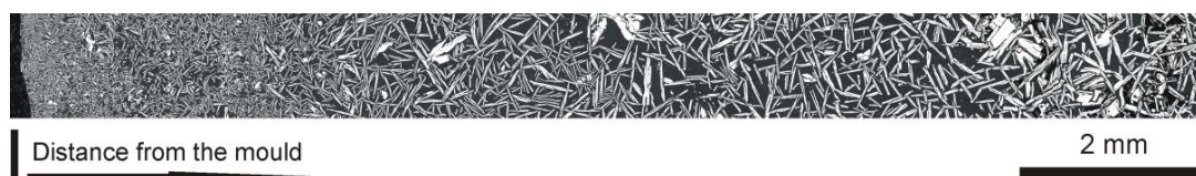
Figure 6. Microstructure evolution with distance from the wall of the mould in the bottom part of the W–Al–VIM-1 ingot.
