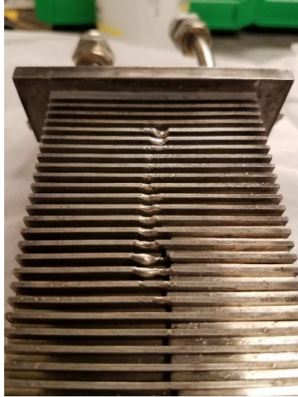
Figure 3.8 – Melt damage on a LiMIT trench module due to 10 \text{ MW/m}^2 e-beam heat flux driving lithium dryout and exposure of the underlying solid substrate [80].
