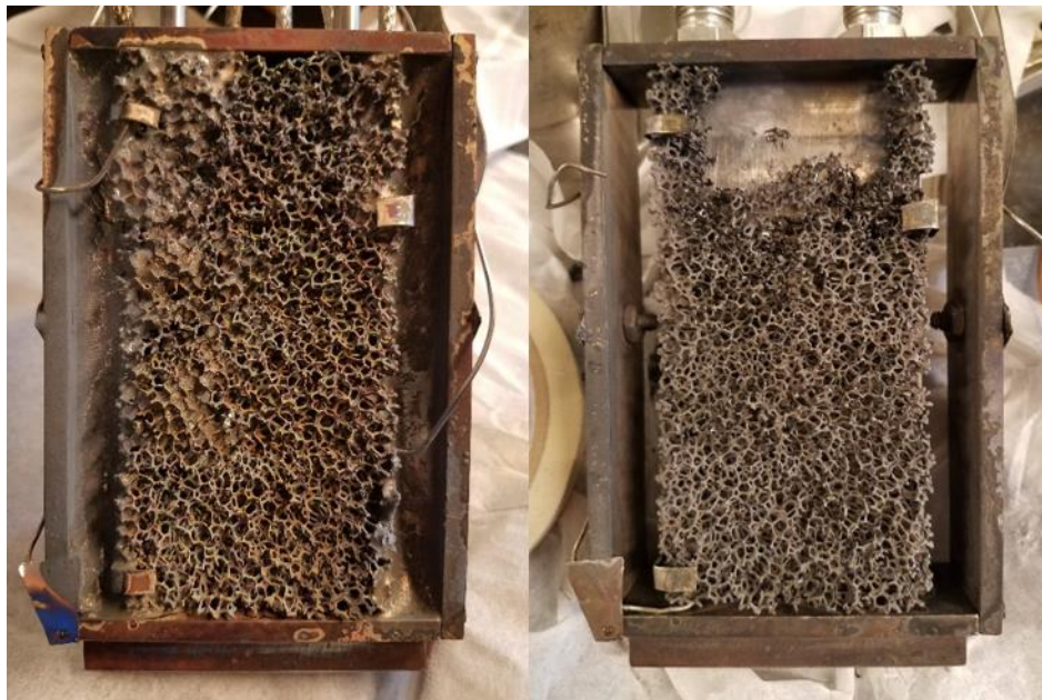
Figure 6.12 – Left: Post-test lithium module with a compromised structure. Right: Partially disintegrated metallic foam after cleaning of lithium.
