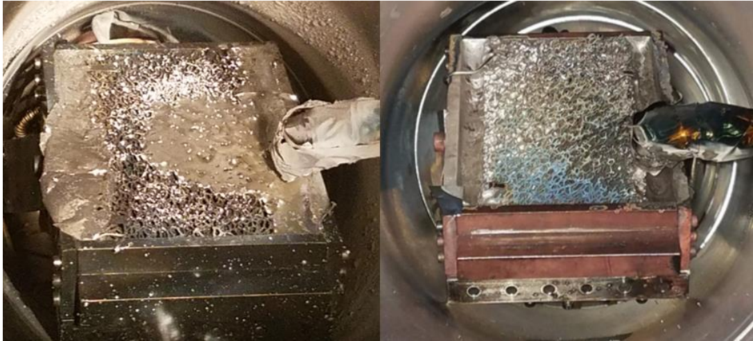
Figure 6.11 – Successful lithium wetting cases in disordered metallic foams. Evidence of impurity layers are seen in the left image, and the right image displays significant lithium underfill.
