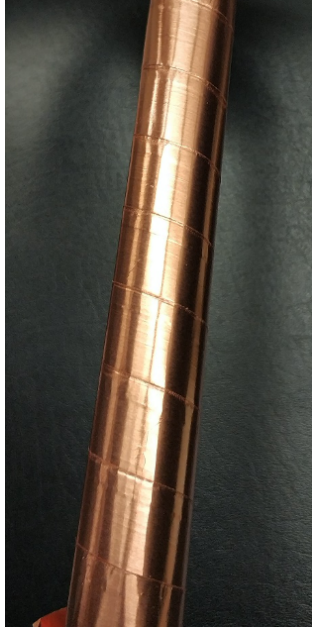
Figure 4.4: Self rolled copper tape with acrylic adhesive on tape. Approximate dimensions are w = 25.4 mm, l = 200 mm, d = 25.4 mm, \theta = 14^\circ , l_0 = 5.4mm
