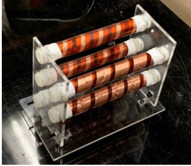
Figure 2.3: HX example using staggered configuration stack of hybrid tubes
