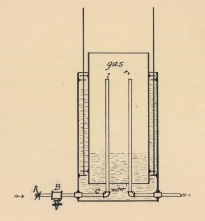
The two tanks were alike, both being made of galvanized iron, except the inner tank for the gas, which was made of tin to make it lighter. As will be seen from the following tests, the temperatures of flue gases at rear end: are very constant, showing that the entrance temperature and quanity of gas are constant.
