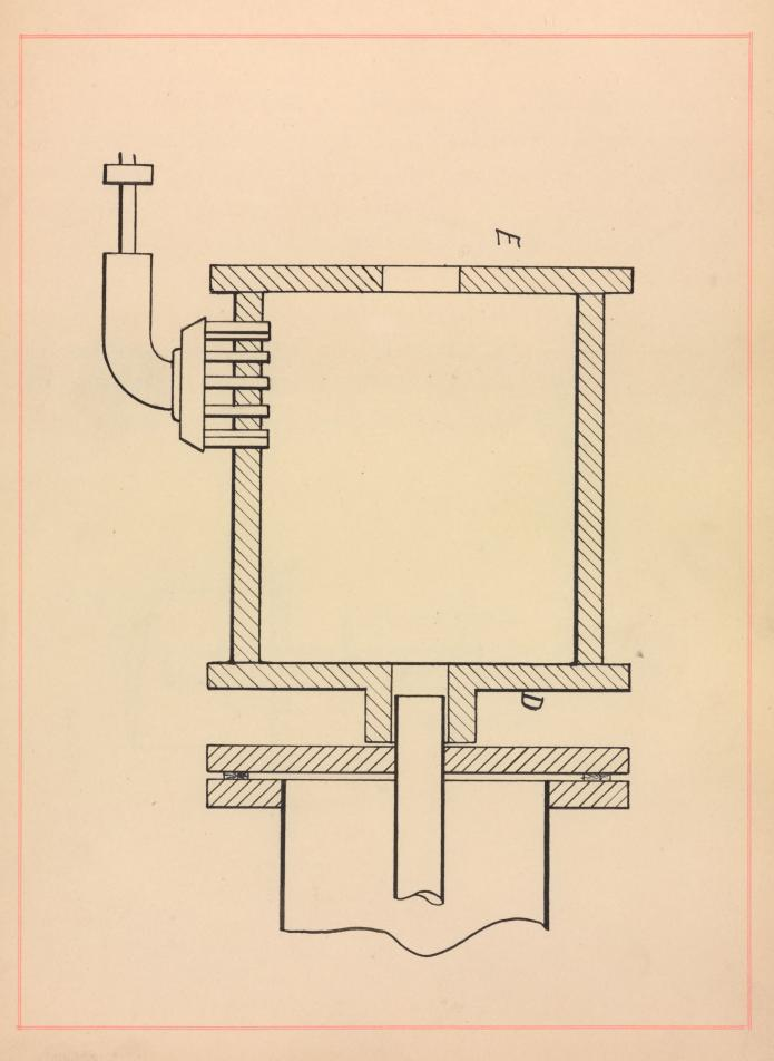
A six inch galvanized iron pipe was made connecting the rear end, B, of the tube to a chimney in the laboatory. It was expected that the hot gases would produce sufficient draft, but on trial failed to make the least sign of any draft.
