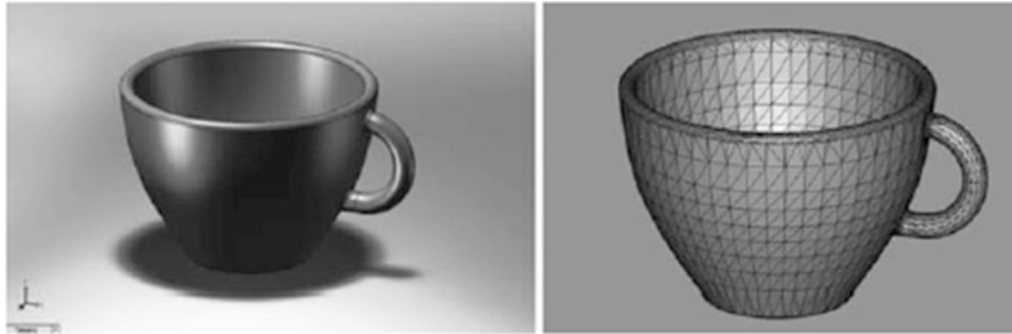
Figure 2.4: An example of a CAD model (left) converted to an STL file (right). Republished with permission of Springer New York, from Gibson et al. (2010); permission conveyed through Copyright Clearance Center, Inc.
