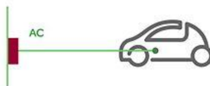
Figure 2.1-4: Mode 1 - fixed, non-dedicated socket [2.19]
