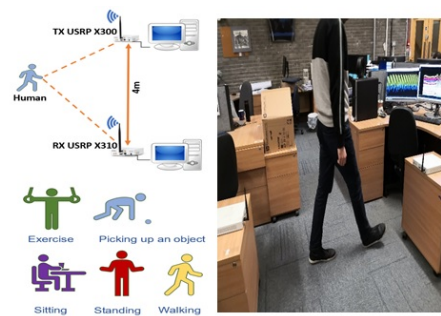
Figure 4. Schematic depiction of experimental setup along with pictorial representation of five different activities classified and actual snapshot of lab environment.
