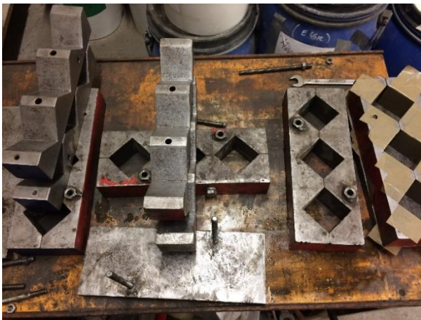
Figure 8: Gang of three 50 mm cube moulds being prepared for use
