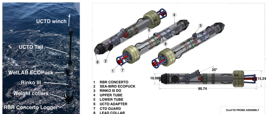
FIG. 1. (left) EcoCTD probe being deployed from the NRV Alliance during a 2018 cruise in the Alboran Sea. (right) Engineering drawing of the EcoCTD design depicting the CTD the key components of the probe. Dimensions are in centimeters unless mentioned otherwise.
