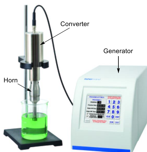
Figure 2.2 Fisher Scientific™ FB-705 Sonic dismembrator components description
