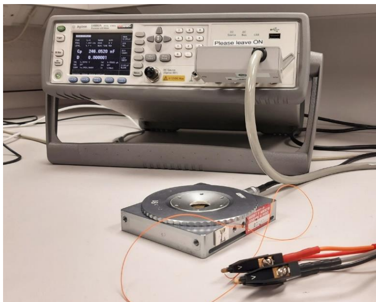
Figure 2.9: The setup for dielectric spectroscopy experiments. The cell is placed on the temperature-controlled hot stage and connected to the spectrometer through the wires.
