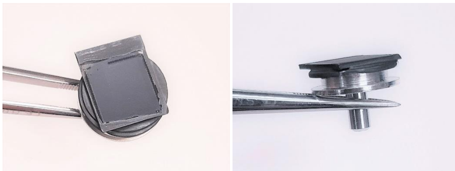
Figure 2.17: Pictures of an SEM sample: a cracked open cell is placed on an aluminium stub and coated with conductive carbon.
