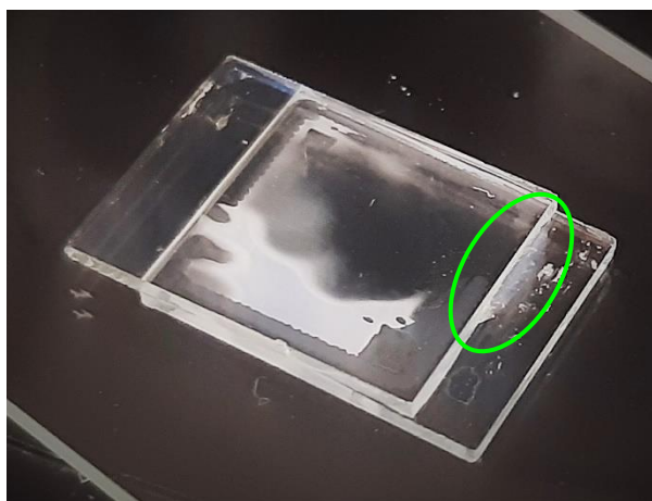
Figure 4.17: The refilling process at room temperature using 5CB: the transparent area represents the template that has been refilled with 5CB, and the white area represents the template that is yet to be refilled. The 5CB liquid crystal is placed at the cell opening (labelled with an oval) and the template is refilled via capillary action.
