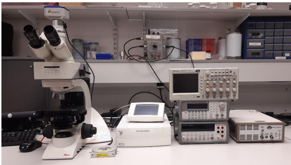
Figure 2.5: The experimental setup for electro-optic experiments: a polarising optical microscope, hot stage, temperature controller and electrical kit.
