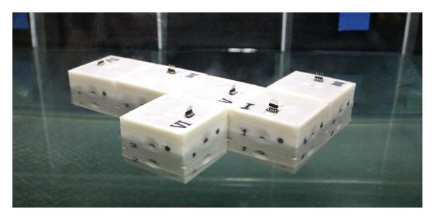
Figure 4.12 The hardware prototype of the MHP system floating on water in a tank. Each module is square shaped and contains four micro-pumps and an internal reservoir, four light sensors, a battery, and a microcontroller.
