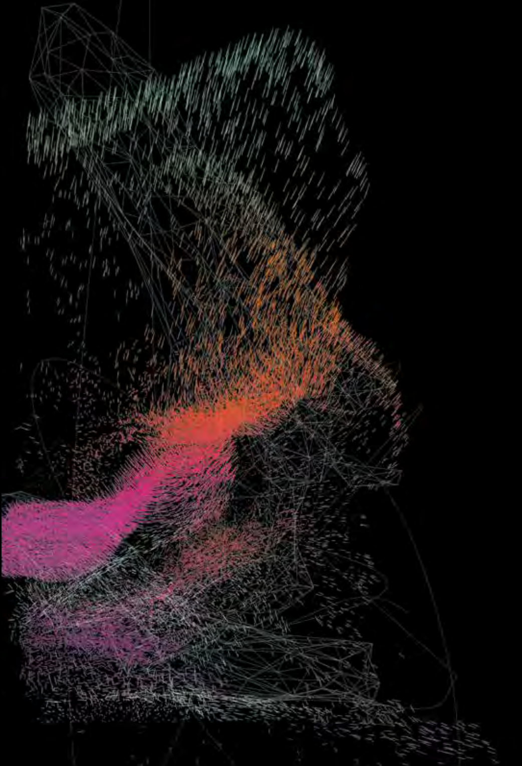
Fig.07. Simulation 2: Erosion + Deposition Simulation looking at the deposition of the soil particles after being transported by the water current. Software: Next Limit: RealFlow.
