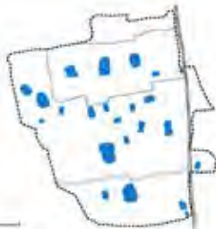
Ground excavated for pukurs, for rainwater collection and fish farming
