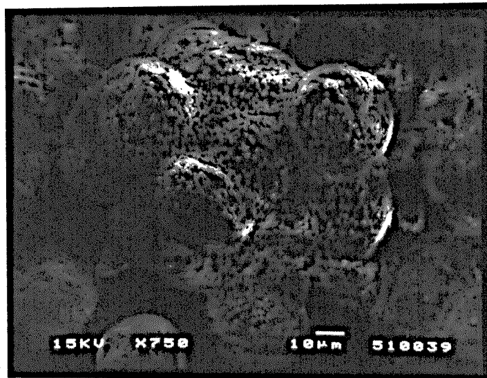
Figure 4.2b SEM photomicrograph showing spherulitic aggregates of scorodite
