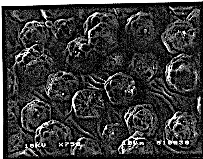
Figure 4.5a SEM photomicrograph showing the nature of the Type-2 compound
