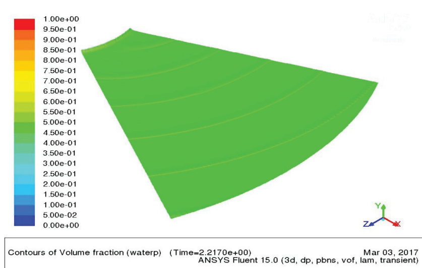
Figure 4.5: Examples of wave structures produced by CFD simulations, with \lambda = 0.02 and r_{disk} = 7
