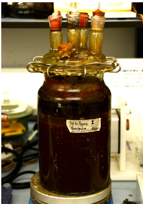
Fig. 5-1 Aerobic batch reactor used to grow nitrifying bacteria, placed in a constant temperature room of 35 °C.
