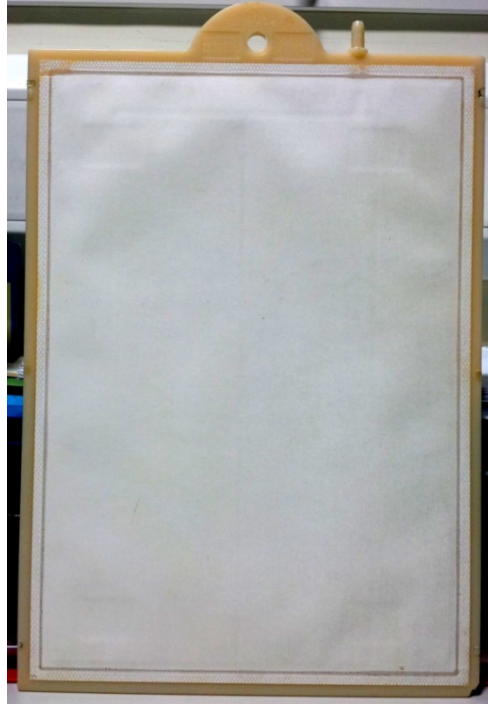
Fig. 3-5 Kubota (type 203) flat panel membrane module used in the SAMBR.
