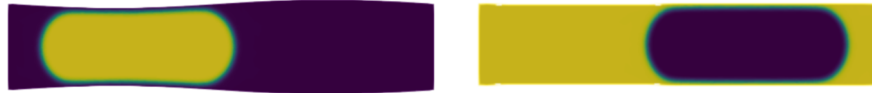
Figure 3.14: Smaller corrugations allow slug flow, the left shows \theta_0 = 140 deg, with the yellow phase appearing to be a slug in blue bulk ( \varepsilon = 0.2 ), the right shows \theta_0 = 40 deg, the blue phase as a slug in bulk yellow phase ( \varepsilon = 0.1 ).
