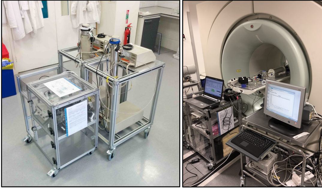
Figure 4.2: Digital photograph of the core-flooding set-up designed and commissioned in this work. The left figure is the experimental system (schematic presented in Figure 4.3) when packed in custom-built trolleys whereas the figure on the right corresponds to the entire set-up placed on the bed of a X-ray CT/PET scanner
